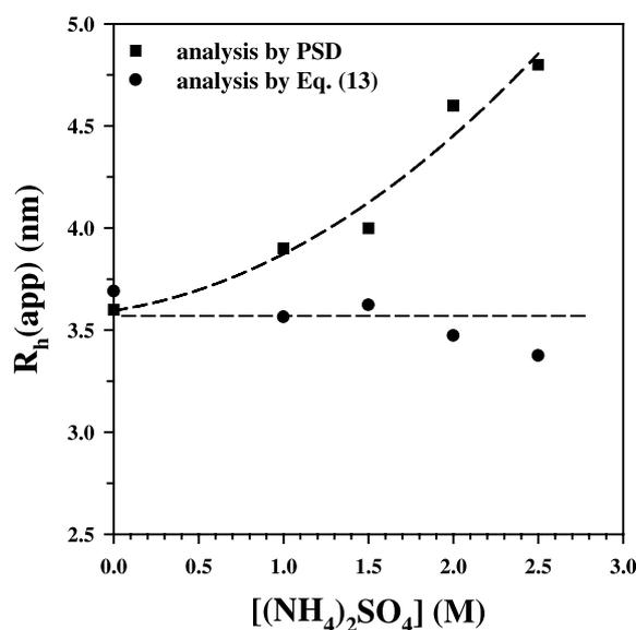
Fig. 1.  $R_h(\text{app})$  versus AS concentration for ESA in 0.1 M NaAc buffer, pH 5.6, 22°C using two methods of data analysis.
