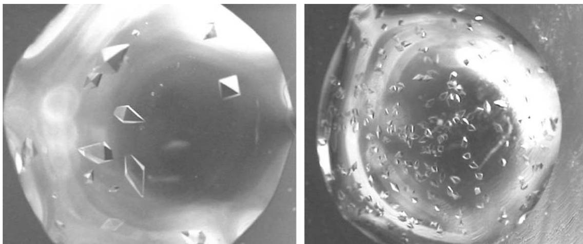
Fig. 4. Thaumatin I crystals grown in 0.5 M ADA buffer, pH 6.5, 22 °C, with 0.75 (left) and 1.0 M (right) NaK tartrate as crystallizing agent and with  $B = -1.8 \times 10^{-4}$  and  $-5.7 \times 10^{-4}$  ( $\text{mol} \cdot \text{ml} \cdot \text{g}^{-2}$ ), respectively.
