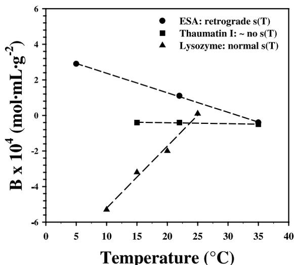
Fig. 5.  $B$  versus temperature for ESA in 0.1 M NaAc buffer, pH 5.6, with 0.5 M AS; thaumatin I in 0.05 M ADA buffer, pH 6.5, with 0.5 M NaK tartrate; and lysozyme in 0.1 M NaAc buffer, pH 4.2, with 2% NaCl (w/v), showing retrograde  $s(T)$ , approximately no  $s(T)$ , and normal  $s(T)$ , respectively.
