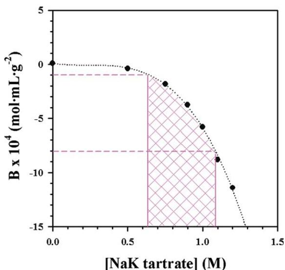
Fig. 3.  $B$  versus NaK tartrate concentration for thaumatin I in 0.05 M ADA buffer, pH 6.5, 22 °C, with crystallization slot overlay.
